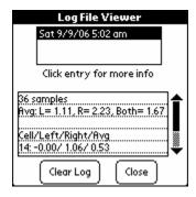
Click the saved entry at the top. Detailed information will be displayed in the bottom part of the screen. Use the scroll bar to the right of this data to page down & see all the collected cell values. The Clear Log button will erase all saved LTrim collections.
